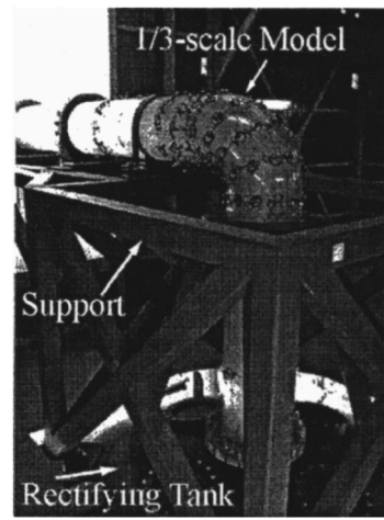
Fig. 3 1/3-scale model pipe installed on the top of the rectifying tank (inner diameter=412.7 mm)
