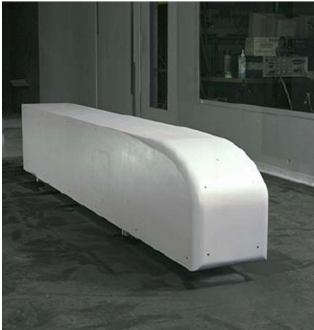
Fig. 1 GTS model in the NASA Ames 7×10 ft wind tunnel (courtesy of Storms et al. [9])
